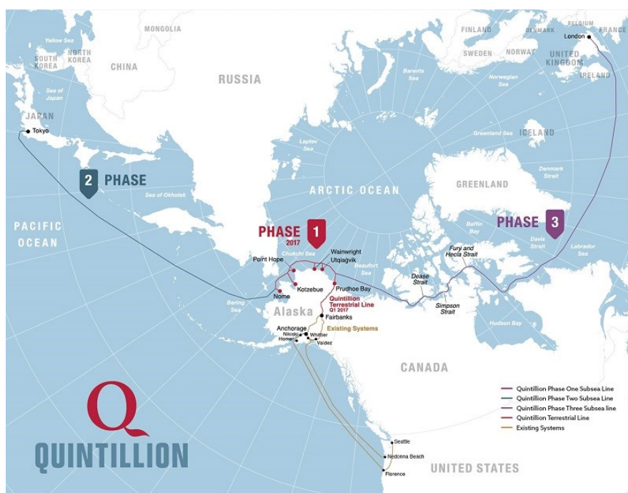
Figure 3.9: Example of Proposed Arctic Submerged Cable through NWP
